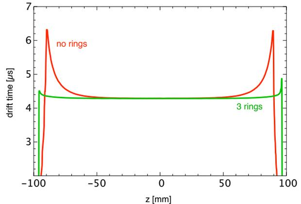
Fig. 3. Drift time of the electrons from the cathode (-500 V) to the anode (0 V) for a 90%Ar/10%  $\text{CO}_2$  gas mixture at STP. Close to the end of the drift region (here at  $z = \pm 100$  mm) the field is too inhomogenous so that only 50% of the drift region could be used. Three voltage supporting rings increase this region to 90%.
