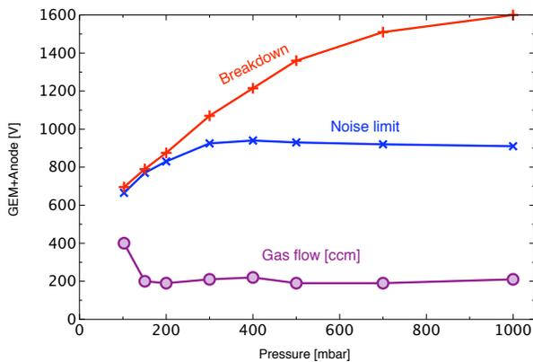
Fig. 1. GEM voltage operating range for different pressure ranges.
