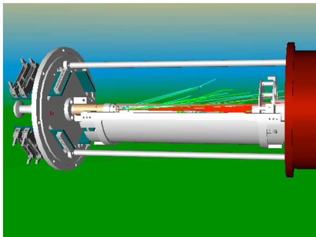
Fig. 4. Sketch of the entire TACTIC. The  $^8\text{Li}$  beam comes from the left and it expands as a solid envelope to the right due to scattering with the target gas in the target region. A few of the  $^8\text{Li}$  and  $^4\text{He}$  tracks make it into the drift region, however most of the tracks in the drift region are from  $^{11}\text{B}$  ions.
