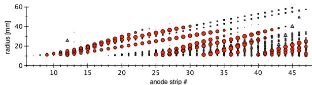
Fig. 2. Simulated ion tracks for the  ${}^8\text{Li}+{}^4\text{He}$  reaction as seen by the 48 anode pads which can detect only electrons from the drift region ( $r = 10\text{--}60$  mm). Circles =  ${}^{11}\text{B}$ , squares =  ${}^8\text{Li}$ , triangles =  ${}^4\text{He}$ . The size of the symbols reflects the energy collected per anode strip.
