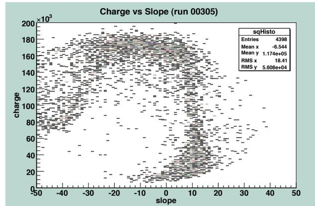
Fig. 5. Integrated charge (arb. units) vs. slope. The slope is the mean time difference (in ns) per strip of an ion track. Positive slope means that the ion moves towards the cathode.
