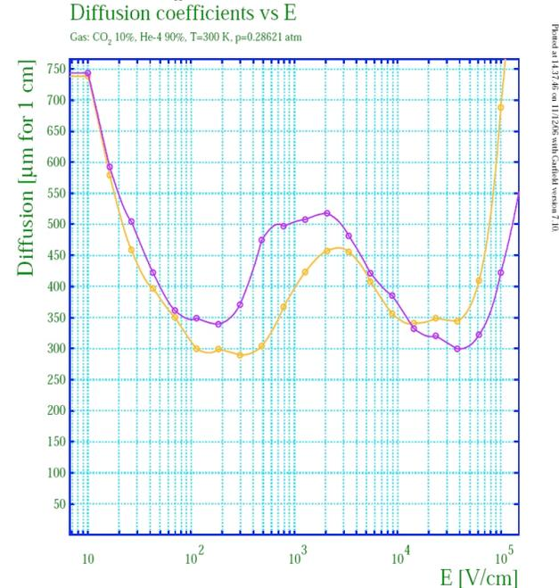
Fig. 2. Longitudinal (yellow) and lateral (purple) diffusion coefficients for a 90% He, 10% CO<sub>2</sub> gas mixture at 290 mb and 300K.
