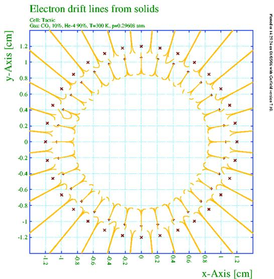
Fig. 1. A Garfield simulation of the TACTIC cathode. The black crosses represent the concentric arrangement of wires, there are 32 in each ring. The inner wires are held at a potential of -1800 V, the outer wires at -2000 V.
