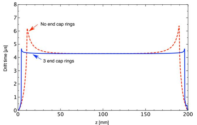
**Fig. 11.** Drift time of electrons released at -500 V biased cathode wires to the GEM vs. the  $z$ -axis, with and without voltage-shaping rings at the end caps at 10 mm radius. The radii of the cathode cage and of the GEM cylinder are 10 mm and 50 mm, respectively.
