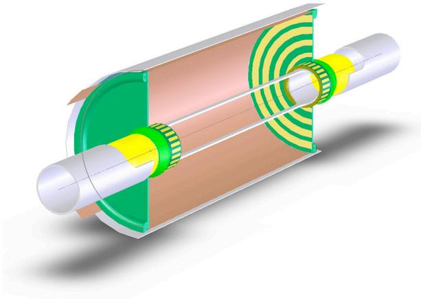
**Fig. 2.** Three-dimensional cut-away view of proposed TACTIC detector.
