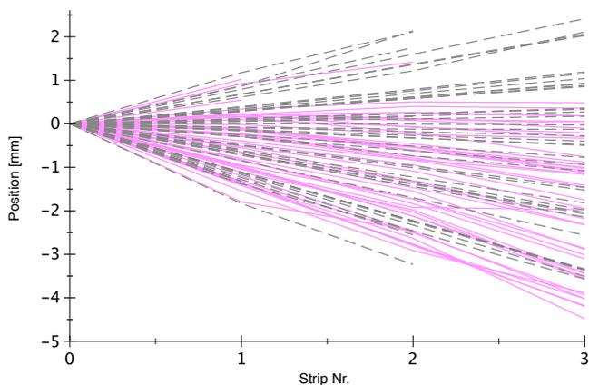
**Fig. 5.** Electron drift times with respect to the first strip, converted to distances assuming a drift velocity of  $12 \text{ mm}/\mu\text{s}$ . The electrons are released along the tracks of the  $\alpha$ 's. The dashed lines stem from a GEANT4 simulation, the solid, purple lines from the measurement.
