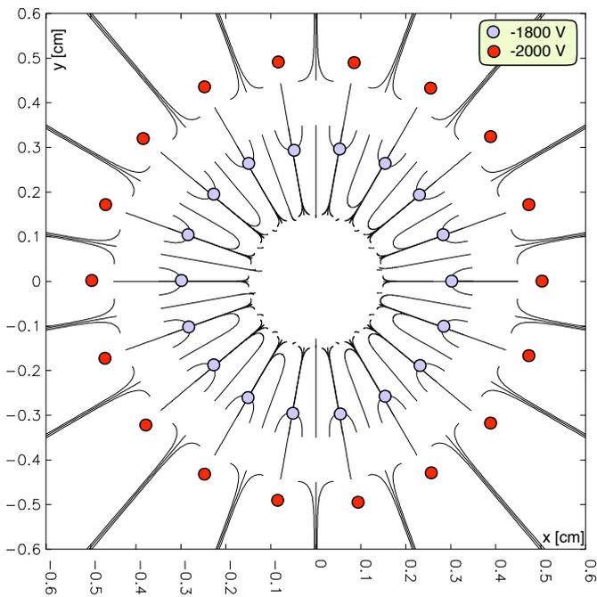
**Fig. 10.** GARFIELD simulation of the electron drift in the target region. The circles mark the wires, and the thin black lines the paths of the electrons released at different positions. Only electrons close to the cathode wire cage reach escape the target region and enter the detection volume.
