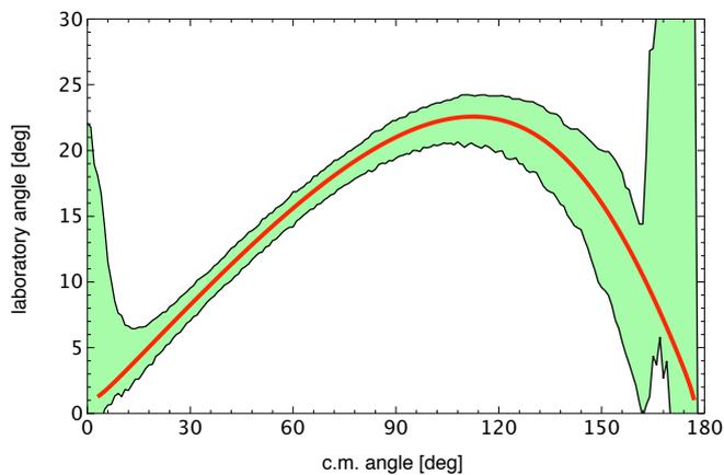
**Fig. 9.** Uncertainty ( $\pm\sigma$  range calculated for 10000 events) of the  $^{11}\text{B}$  laboratory angles, reconstructed using 48 anode rings, each 5 mm in width, emitted at different c.m. angles as expected from the GEANT4 simulation for the  $^{11}\text{B}$  ground state. Overlaid is the theoretical curve.
